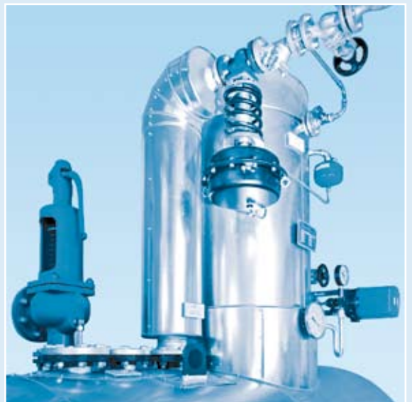
e.g. feedwater tank with deaerator dome... ... for supplying returned condensate and fresh water to the boiler via the deaerator dome and the feed water tank. The exceptionally durable design of the boiler is achieved by removing inert gases from the condensate / fresh water.
